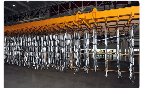
Transfer. Once cool, products are taken off the line for inspection and packing ( P10 ).
