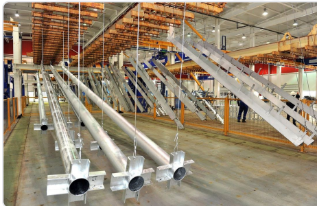
07 — Cooling. Parts are cooled on the jig without touching each other; a contact point leaves a mark in the coating.
