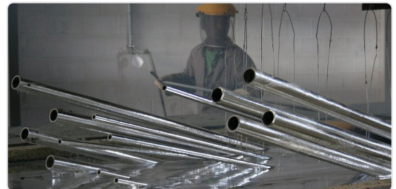
Parts are hung individually and dipped without touching each other. The open mesh of a grating helps the zinc drain.
