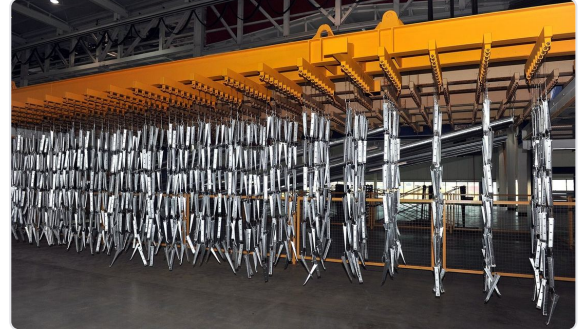
Galvanized products are taken off the line once cool; final inspection and packing start here.
